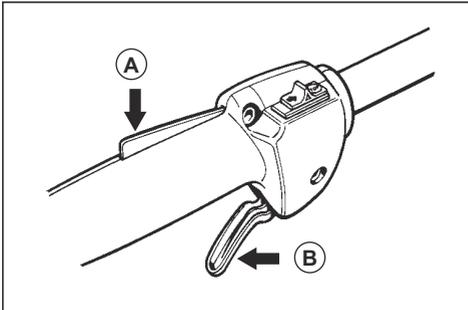
2. Release the throttle trigger lockout and make sure that the throttle control is locked at idle speed.
