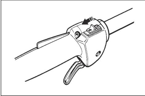
2. Set the choke control to the choke position.
