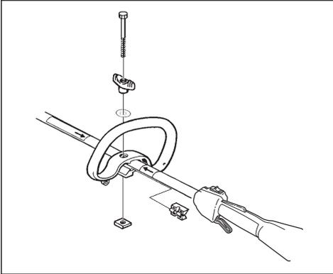
2. Put the spacer into the slot of the loop handle.
