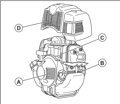
1. Clean the cooling system with a brush weekly or more frequently if it is necessary.
