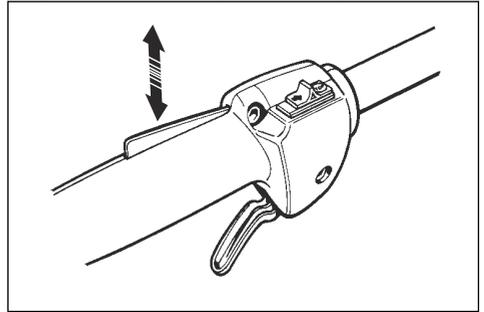
4. Make sure that the throttle control and throttle trigger lockout move freely and that the return springs operate correctly.
