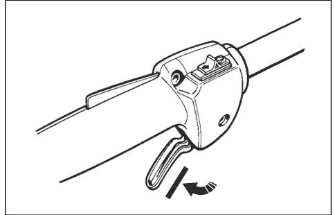
3. Push the throttle trigger lockout and make sure that it goes back to its initial position when you release it.
