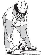
Push in the choke control as soon as the engine fires and keep pulling until the engine starts. When the engine starts, quickly apply full throttle; the throttle start lock will automatically disengage.
