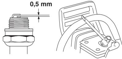
Note! Always use the recommended spark plug type! Use of the wrong spark plug can damage the piston/cylinder. Check that the spark plug is fitted with a suppressor.
