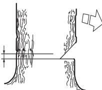
Set the spike bumper (if one is fitted) just behind the felling hinge. Use full throttle and advance the chain/bar slowly into the tree. Make sure the tree does not start to move in
