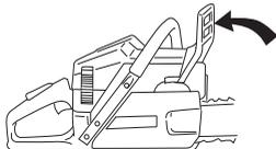
Remove the bar nuts and remove the clutch cover (chain brake). Take off the transportation ring (A).
