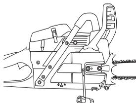
The chain is correctly tensioned when it does not sag from the underside of the bar, but can still be turned easily by hand. Hold up the bar tip and tighten the bar nuts with the combination spanner.
