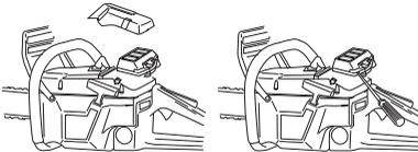
The filter can be cleaned more thoroughly by washing it in water and detergent.
