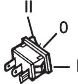
The switch is off in position "0", supplies current to the handle heater in position "I", supplies current to the carburettor in position "II".
