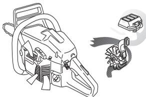
**IMPORTANT!** In order to maintain operation of the centrifugal cleaning system it must be regularly maintained. Clean the air intake to the starter, the fins on the flywheel, the space around the flywheel, inlet pipe and carburettor compartment.
