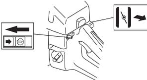
If the machine is fitted with a decompression valve (A): Press the valve to reduce the pressure in the cylinder and make starting easier. You should always use the decompression valve when starting the machine. Once the machine has started the valve will automatically return to its original setting.
