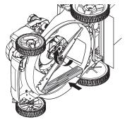
5 The bolt should be tightened with a torque of 35-40 ft. lbs. / 47-54 Nm. 6 Verify the spark plug wire is disconnected from the engine.
