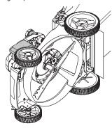
4 Use a wood block between blade and mower housing to prevent blade from turning when removing blade bolt.
