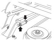
4 Screw out (extend) the stay to raise the rear edge of the cover.
