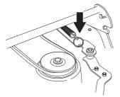
6 Lift off the drive belt and hang on the load-relieving hook.
