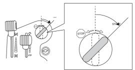
6 When the engine starts release the ignition key immediately back to neutral position.
