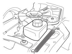
3 Fill if necessary with engine oil SAE 10W/40 (class SF-CC).
