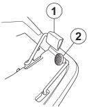
3 Select the required cutting height (1-10) with the cutting height lever.
