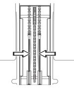
3 If necessary, the wires can be adjusted by tightening the adjuster nuts on each side of the steering collar. Do not over tighten the cables; they should only be drawn in towards the steering collar.
