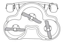
CAUTION! One or more unbalanced blades , caused by damage or poor balancing after sharpening, can cause vibrations in the machine.
