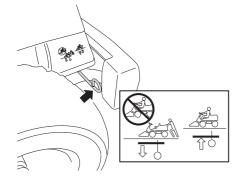
2 Lift up the cutting unit by pulling the lever backwards to locked position (transport position) and apply the parking brake. The engine can not be started if the parking brake is not pressed down.
