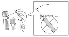
3 When the Rider is at a standstill, press down the parking brake and push in the locking button.
