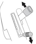
2 Release the clip on the front hood and lift off the fender.
