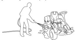
**IMPORTANT INFORMATION** Always park the machine on a level surface with the engine OFF before performing any maintenance.
