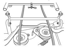
Make sure the lifting lever comes above the cutting deck grip.
