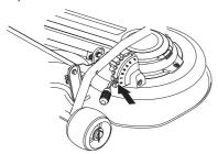
4 Put the lifting lever in the mowing position.
