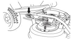
4 Fit the cutting deck's pipe together with the deck frame's pipe.
