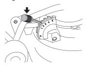
In order to obtain an even cutting height, it is important that the air pressure is the same in both front wheels. See the "Technical data" section.
