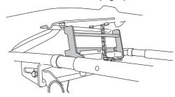
2 Place the belt under the stay of the cutting deck.
