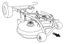
12 Lift off the deck and lean it against the machine or a wall.
