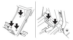
2 Check the tension of the steering wires by squeezing them together by the arrows as illustrated.
