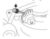
Lift up the cutting unit before adjusting the height.
