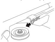
11 Loosen the stay from the cutting deck.
