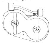
The blades should be balanced after sharpening.
