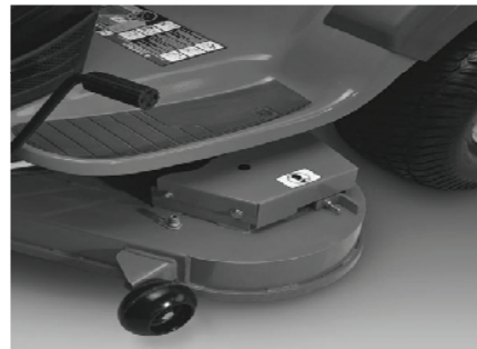
Fabricated Deck Shell Example Below
