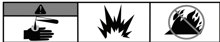
Battery acid is corrosive, explosive and flammable
