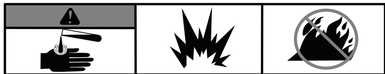
Battery acid is corrosive, explosive and flammable
