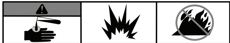
Battery acid is corrosive, explosive and flammable
