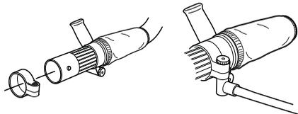
Assemble the intermediate pipe.
