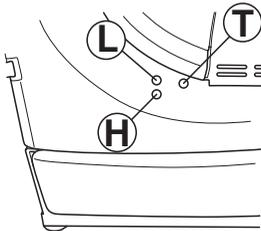
The L and H-jets are used to adjust the supply of fuel to match the rate that air is admitted, which is controlled with the throttle. If they are screwed clockwise the air/fuel ratio becomes leaner (less fuel) and if they are turned anti-clockwise the ratio becomes richer (more fuel). A lean mixture gives a higher engine speed and a rich mixture gives a lower engine speed.
