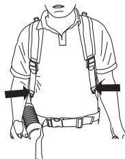
Place the hip strap over the hip and not too far down on the stomach. Tighten the hip strap so that you feel the weight of the blower resting on your hip.
