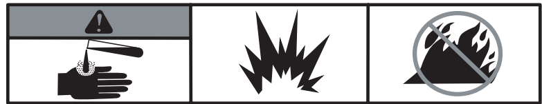
Battery acid is corrosive, explosive and flammable
