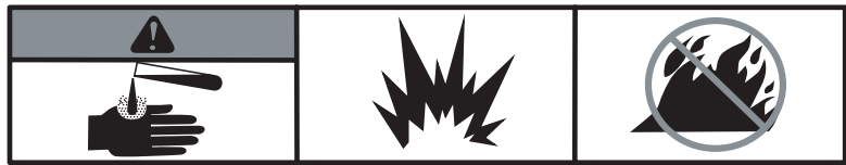
Battery acid is corrosive, explosive and flammable
