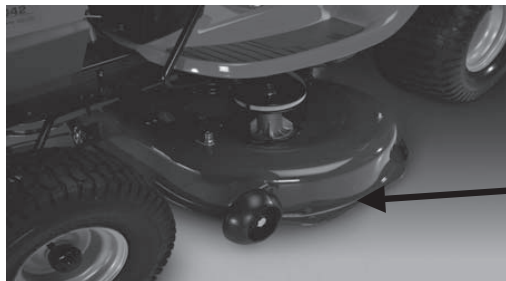
Stamped Deck Shell below, NOT reinforced
