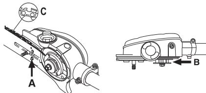
Tension the chain by turning the chain tensioning screw clockwise using the combination spanner. The chain should be tensioned until it does not sag from the underside of the bar.
