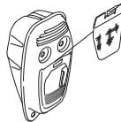
On mufflers without a catalytic converter the mesh should be cleaned weekly, or replaced if necessary. On mufflers fitted with a catalytic converter the mesh should be checked, and if necessary cleaned, monthly. **If the mesh is damaged it should be replaced.**
