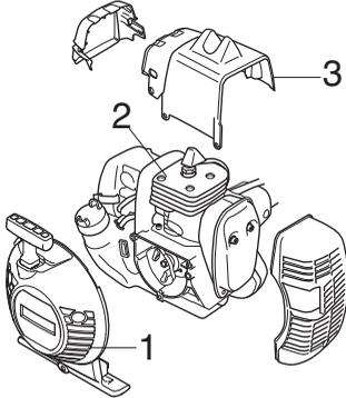
The cooling system consists of:
