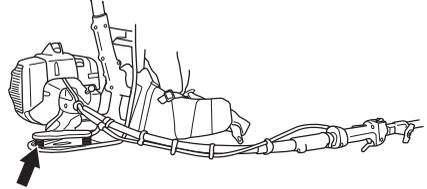
The machine's vibration damping system reduces the transfer of vibrations.
