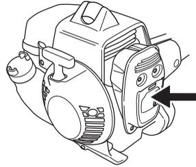
Some mufflers are equipped with a special spark arrester mesh. If your machine has this type of muffler, you should clean the mesh at least once a week. This is best done with a wire brush.
