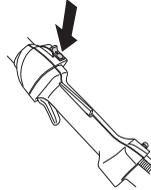
Start the engine and make sure the engine stops when you move the stop switch to the stop setting.
