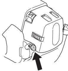
**Choke:** Set the choke control in the choke position.
