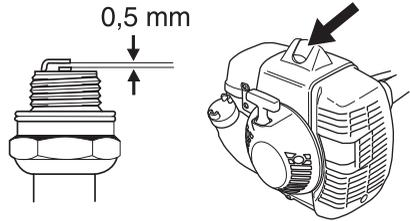
**CAUTION!** Always use the recommended spark plug type! Use of the wrong spark plug can damage the piston/cylinder. Check that the spark plug is fitted with a suppressor.
