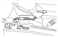
4 Select the required cutting height (1-10) with the cutting height lever.
