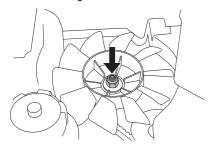
5 Check that the centre belt is fitted correctly on its front pulley and fit the centre belt on the engine's pulley.
