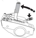
3 Remove the front hood by removing the pin. (There are complete instructions on using the service position inside the front hood).
