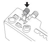
Set the required engine speed with the throttle control.
