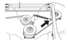
Simply reverse the procedure to fit the new belt.
