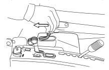
Secure the cutting unit if necessary using the mechanical lifting lever.
