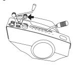
For cold starting the lever is moved backwards to its end position.
