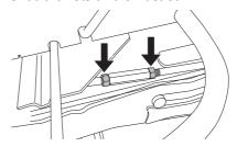
3 Screw out (extend) the stay to raise the rear edge of the cover.
