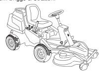
The machines are equipped with power steering and hydraulic lifts. R 422 Ts AWD also have all wheel drive.
