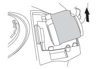
4 Remove the foam rubber prefilter which is placed around the filter cartridge and clean using a mild detergent. Squeeze it dry in a clean cloth.
