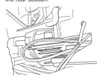
6 Remove the cooling fan, it is held in place by a nut.
