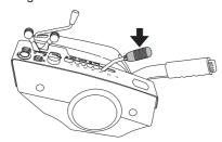
It is important that the air pressure in both front wheels is equal, 60 kPa  $\!\!/$  0,6 bar  $\!\!/$  8.7 PSI, to produce an even cutting height.
