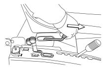
In order to ensure that the hydraulic cylinder is in the outer position, hold the lever in the forward position for a half to one second
