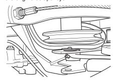
8 Pull out the belt through the opening under the pivot bearing and past the belt tensioner's disc.
