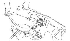
7 Loosen the spring that tensions the V-belt and pry off the belt.
