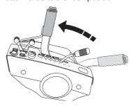
If the cutting unit is left in the lower position, the start lock circuit will prevent engine starts.
