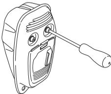
If the muffler on your machine is fitted with a spark arrestor mesh this must be cleaned regularly. A blocked
