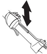
Check that the throttle control and throttle lockout move freely and that the return springs work properly.
