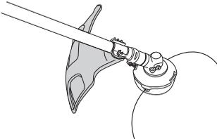
Check that the guard is undamaged and not cracked. Replace the guard if it has been exposed to impact or is cracked.
