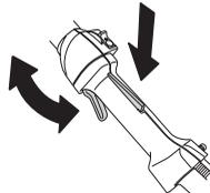
See instructions under the heading Start. Start the machine and apply full throttle. Release the throttle and check that the cutting attachment stops and remains at a standstill. If the cutting attachment rotates with the throttle in the idle position then the carburettor idle setting must
