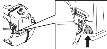
**Choke:** Set the choke control in the choke position.
