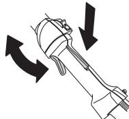
See instructions under the heading Start. Start the harvesting equipment and apply full throttle. Release the throttle trigger and check that the blades stop and remain stationary. If the shaft move when the throttle trigger is in the idle position then the carburettor idle setting must be adjusted. See instructions under the heading Maintenance.
