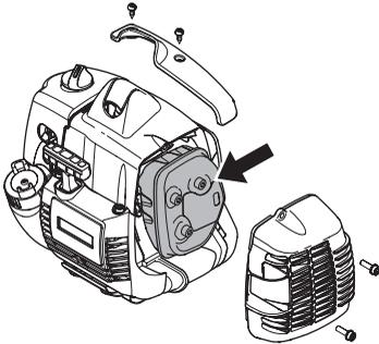
Some mufflers are equipped with a special spark arrestor mesh. If your machine has this type of muffler, you should clean the mesh at least once a week. This is best done with a wire brush.
