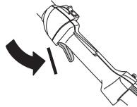
Press the throttle lockout and make sure it returns to its original position when you release it.
