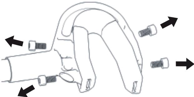
Remove the damaged rubbers and take off the metal nuts located inside of the rubber.
