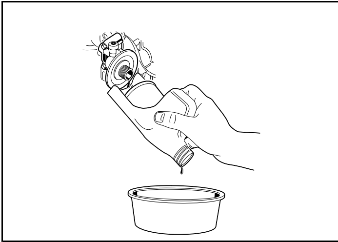
Figure 23 Remove Engine Oil Filter
