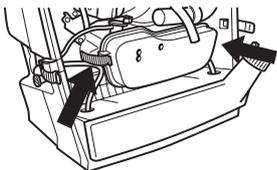
The air filter is fitted in the air filter cowling.
