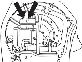
Pull out the spark arrestor screen and clean using a wire brush. Replace the spark arrestor screen if it is defective.
