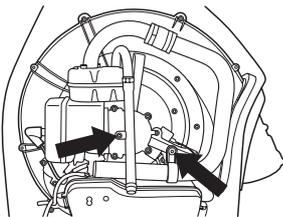
Loosen the muffler's 2 screws and remove the muffler.
