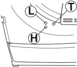
The L and H-jets are used to adjust the supply of fuel to match the rate that air is admitted, which is controlled with the throttle. If they are screwed clockwise the air/fuel ratio becomes leaner (less fuel) and if they are turned anti-clockwise the ratio becomes richer (more fuel). A lean mixture gives a higher engine speed and a rich mixture gives a lower engine speed.
