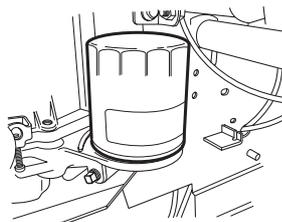
Lightly lubricate the rubber seal on the new oil filter using new oil. Fit the oil filter by turning clockwise. Turn by hand until the rubber seal is seated. Now tighten a further half turn.
