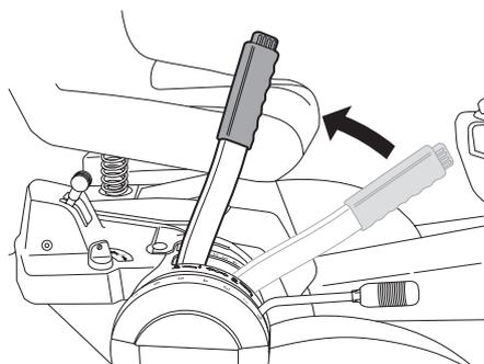
Rider 155 AWD The engine can not be started if the parking brake is not pressed down.
