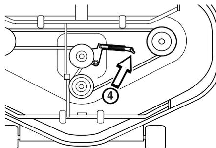
Simply reverse the procedure to fit the new belt.
