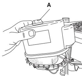
Carefully remove the precleaner. Wash and oil the precleaner every 25 hours of operation. Wash the precleaner in warm water with detergent. Rinse precleaner with clear warm water. Squeeze water out (do not wring to avoid tearing). Allow to dry before lightly oiling with fresh engine oil and installing it over the paper filter.
