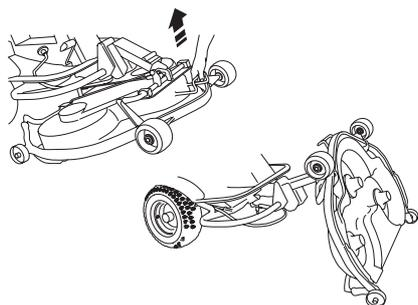
If the cylindrical bolt, which is now holding the cutting unit is removed, the cutting unit can be lifted off.
