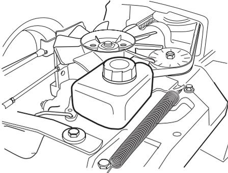
**Rider 155** Fill if necessary with engine oil SAE 10W/30 (class SF-CC).
