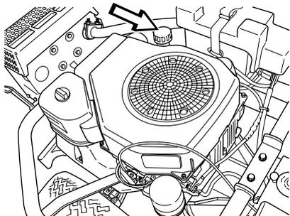
Now insert the dipstick again. The dipstick should be **completely screwed down**
