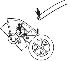
Position the bevel gear so that the slot aligns with the line on the shaft.
