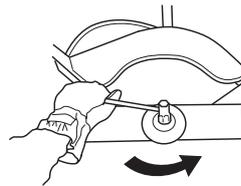
When fitting, tighten the nut in the opposite direction to the direction of rotation of the cutting attachment. To remove it, undo the nut in the same direction as the cutting attachment rotates. (CAUTION! The nut has a left-hand thread.)
