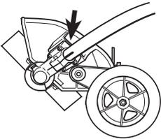
Firmly tighten the screw.
