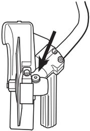
The grease in the bevel gear does not normally need to be changed except if repairs are carried out.
