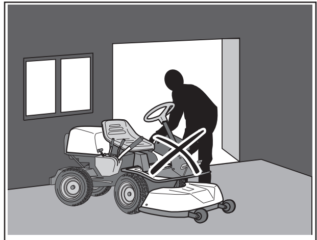
Never fill the fuel tank indoors.
