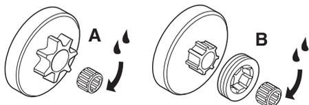
Both versions have a needle bearing on the drive shaft, which has to be greased regularly (once a week).
