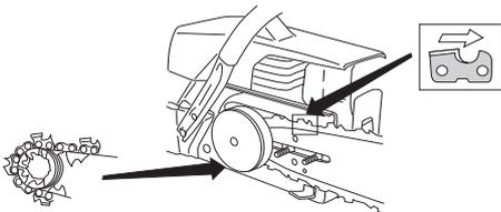
Make sure that the edges of the cutting links are facing forward on the top edge of the bar.
