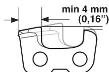
When the length of the cutting teeth has worn down to only 4 mm the chain must be replaced.
