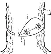
All control over the felling direction is lost if the felling hinge is too narrow or non-existent, or if the directional cuts and felling cut are badly placed.
