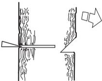
Finish the felling cut parallel with the directional cut line so that the distance between them is at least 1/10 of the trunk diameter. The uncut section of the trunk is called the felling hinge.
