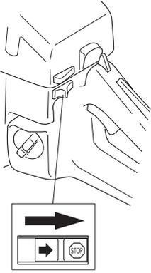
Stop the engine by switching off the ignition. (Move the ignition switch to stop position.)
