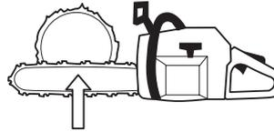
Finish by cutting from above so that the two cuts meet.
