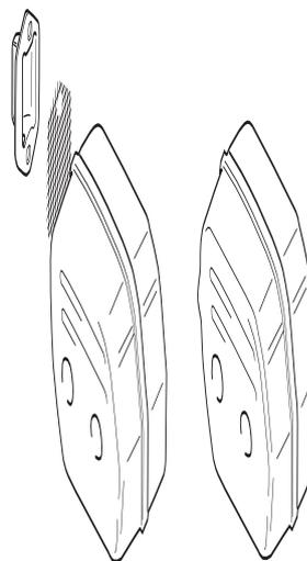
Some mufflers are equipped with a special spark arrestor mesh. If your machine has this type of muffler, you should clean the mesh at least once a week. This is best done with a wire brush.
