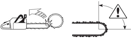
Kickback always occurs in the cutting plane of the bar. Normally the chain saw and bar are thrown backwards and upwards towards the user. However, the chain saw may move in a different direction depending on the way it was being used when the kickback zone of the bar touched the object.
