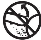
Tip contact may cause the guide bar to move suddenly upward and backward, which may cause serious injury. Please see pages 12-21 in your "Chain saw operator's safety manual".
