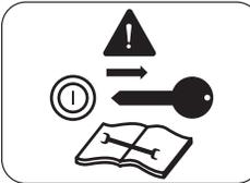
Shut off engine & remove key before performing any maintenance or repair work.
