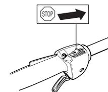
**CAUTION!** The stop switch automatically returns to the start position. In order to prevent unintentional starting, the spark plug cap must be removed from the spark plug when assembling, checking and/or performing maintenance.
