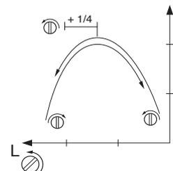
**CAUTION!** If the blades move while the engine is idling the T screw should be turned anti-clockwise until they stop.
