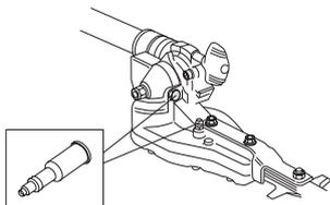
**CAUTION!** The gear housing must not be filled completely with grease. The grease expands as the machine heats up during operation. If the gear housing was completely filled with grease it could damage the seals and lead to leakage of grease.
