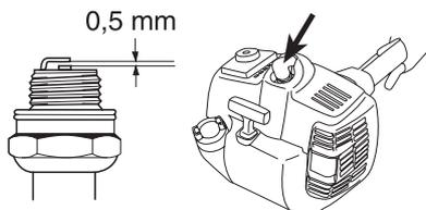
**CAUTION!** Always use the recommended spark plug type! Use of the wrong spark plug can damage the piston/cylinder. Check that the spark plug is fitted with a suppressor.
