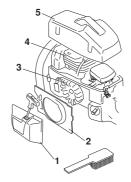
Clean the cooling system with a brush once a week, more often in demanding conditions. A dirty or blocked cooling system results in the machine overheating which causes damage to the piston and cylinder.
