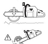
If it is possible (can you turn the log?) stop cutting about 2/3 of the way through the log.
