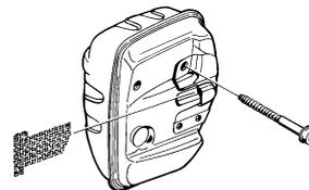
On mufflers without a catalytic converter the mesh should be cleaned weekly, or replaced if necessary. On mufflers fitted with a catalytic converter the mesh should be checked, and if necessary cleaned, monthly. **If the mesh is damaged it should be replaced.**
