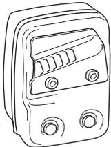
In countries that have a warm and dry climate there is a significant risk of fire. We therefore fit certain mufflers with a spark arrestor mesh. Check whether the muffler on your machine is fitted with this kind of mesh.
