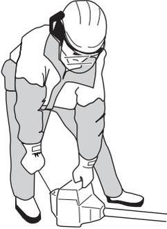
CAUTION! Do not pull the starter cord all the way out and do not let go of the starter handle when the cord is fully extended. This can damage the machine.
