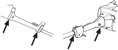
The machine's vibration damping system reduces the transfer of vibration between the engine unit/cutting equipment and the machine's handle unit.
