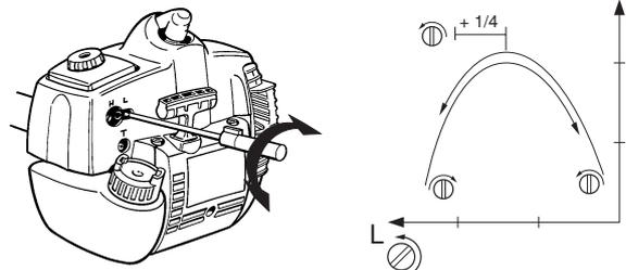
**CAUTION!** If the cutting attachment rotates when the engine is idling the idle adjustment screw T should be turned anti-clockwise until the cutting attachment stops.
