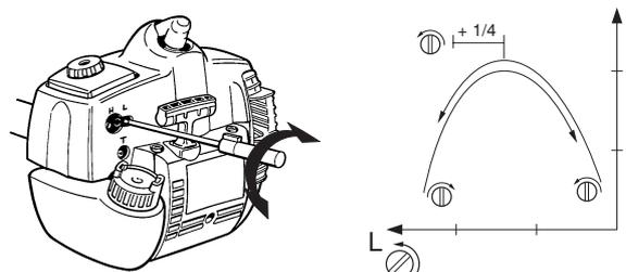
**IMPORTANT!** If the idle speed cannot be adjusted so that the cutting attachment stops, contact your dealer/service workshop. Do not use the machine until it has been correctly adjusted or repaired.
