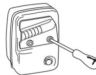
If the muffler on your machine is fitted with a spark arrestor mesh then it should be cleaned regularly. A blocked mesh causes the engine to overheat, which can lead to serious damage.
