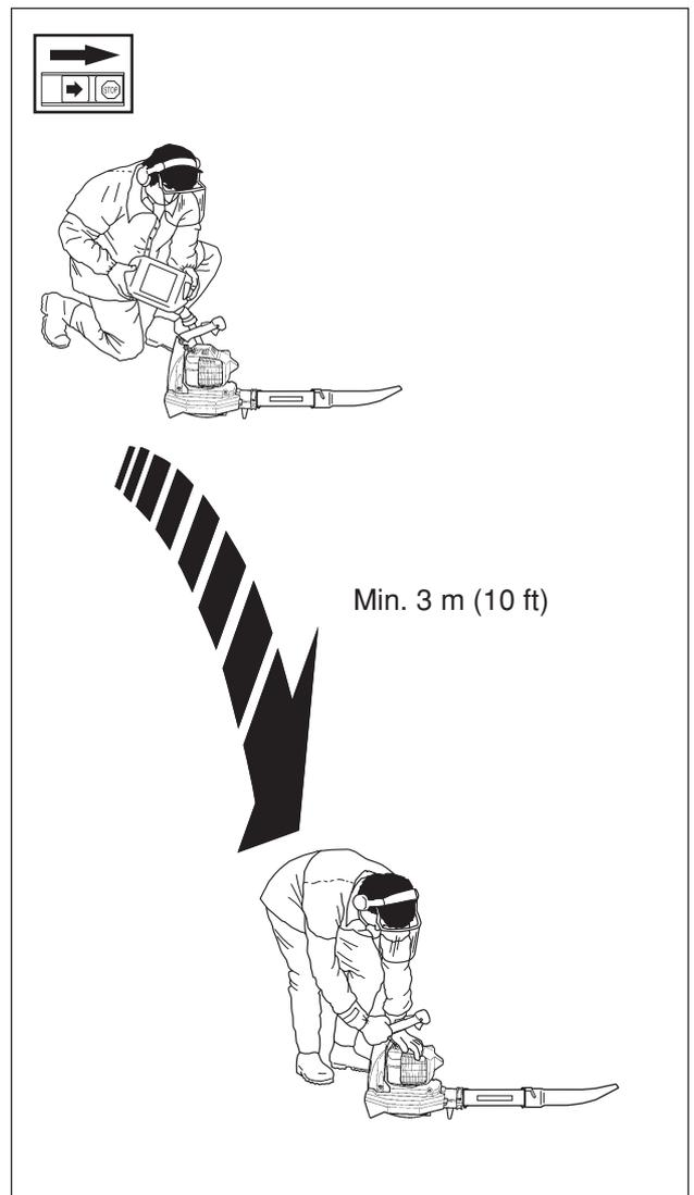
Diagram illustrating fuelling precautions. It shows a person fuelling a chainsaw and a safety distance of 3 meters (10 ft) between the fuelling area and the machine.
