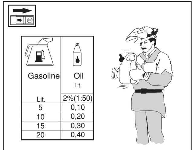
Diagram illustrating fuel mixing instructions. It includes a table for Gasoline and Oil quantities, and an illustration of a person shaking a fuel container.
