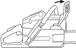
**Starting:** The chain brake must be engaged when the chain saw is started. Activate the brake by moving the front hand guard forwards.
