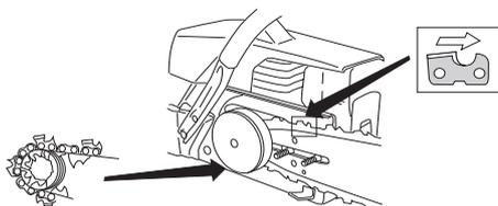
Make sure that the edges of the cutting links are facing forward on the top edge of the bar.
