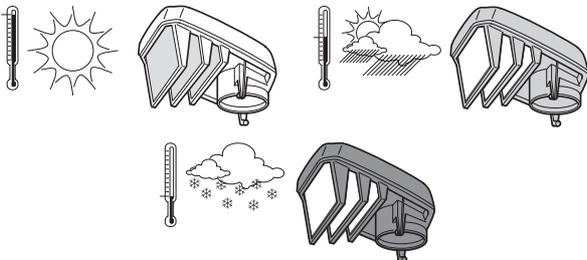
An air filter that has been in use for a long time cannot be cleaned completely. The filter must therefore be replaced with a new one at regular intervals. **A damaged air filter must always be replaced.**
