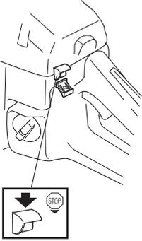
Stop the engine by switching off the ignition.
