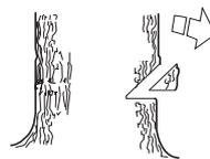
The directional cuts should run 1/4 of the diameter through the trunk and the angle between the top cut and bottom cut should be 45°.
