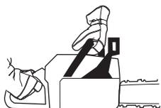
Apply full throttle and activate the chain brake by tilting your left wrist forward onto the hand guard. Do not let go of the front handle. **The chain should stop immediately.**
