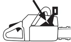
Move the hand guard forwards and back to make sure it moves freely and that it is securely anchored to the clutch cover.
