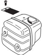
Never use a muffler if the spark arrestor mesh is missing or defective.
