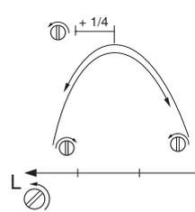
Try to find the highest idle speed by turning the low speed jet L clockwise then anti-clockwise. When the highest speed has been found, turn the low speed jet L 1/4 turn anti-clockwise.
