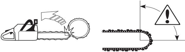
Cutting with the bottom edge of the bar, i.e. from the top of the object downwards, is known as cutting on the pull stroke. In this case the chain saw pulls itself towards the tree and the front edge of the chain saw body rests naturally on the trunk when cutting. Cutting on the pull stroke gives the operator better control over the chain saw and the position of the kickback zone.
