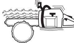
Cutting hardwoods (most broadleaf trees) creates more vibration than cutting softwoods (most conifers). Cutting with cutting equipment that is blunt or faulty (wrong type or badly sharpened) will increase the vibration level. See instructions under the heading Cutting equipment.
