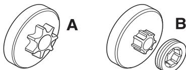
Regularly check the degree of wear on the drive sprocket. Replace if wear is excessive. Replace the drive sprocket whenever you replace the chain.
